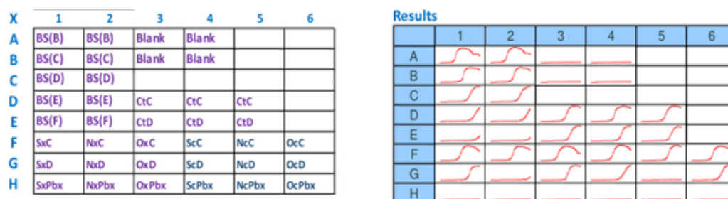
Fig. 5.17: Left part: scheme of experiment. Silica surfaces are indicated with S, etched titanium discs are indicated with O and non-etched ones with N. Ubx-coated surfaces are indicated with 'x', while control surfaces are indicated with 'c'. On the top of samples bacteria solutions, C and D, and plain PBS (indicated as PBX) were pipetted. Right part: results of overnight fluorescence.
