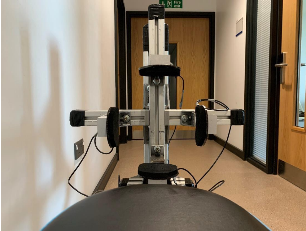
Figure 5: End-on view showing the head piece with load cells, also visible is the horizontal bench where the participant's torso will be strapped down
