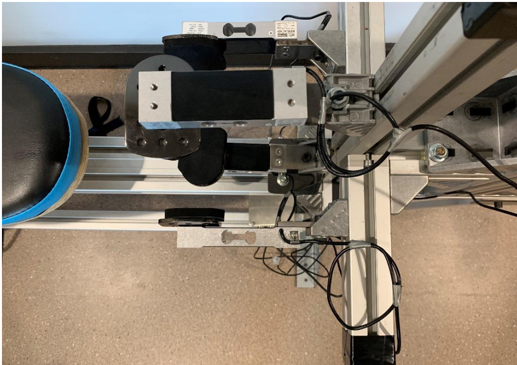
Figure 4: Top view of the head piece, showing the brackets used to fix load cells to the head piece
