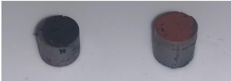
Figure 7.12. Images of \text{Fe}_2\text{O}_3\text{-FC} (left) and \text{Fe}_2\text{O}_3\text{-C} (right) briquettes reduced at 650 °C for 1 hr under \text{N}_2 .
