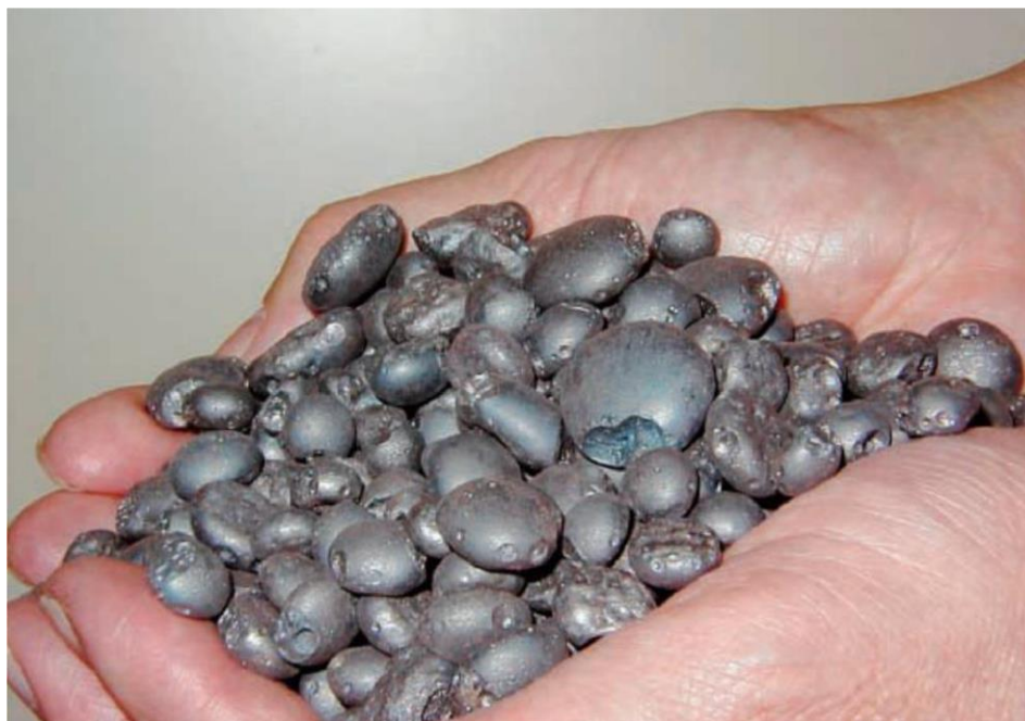
Figure 6.1. Iron nuggets produced via a large scale ITmk3 pilot plant 82 . Reproduced with permission from the Kobe Steel Engineering Report Editorial Board.
