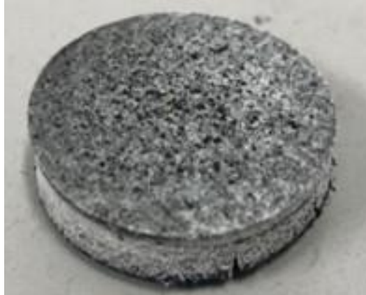
Figure 5.11. Fired pellet (1100 °C, 0 min, C/O = 0.5) removed and quenched from furnace showing white powder layer condensed onto pellet surface.
