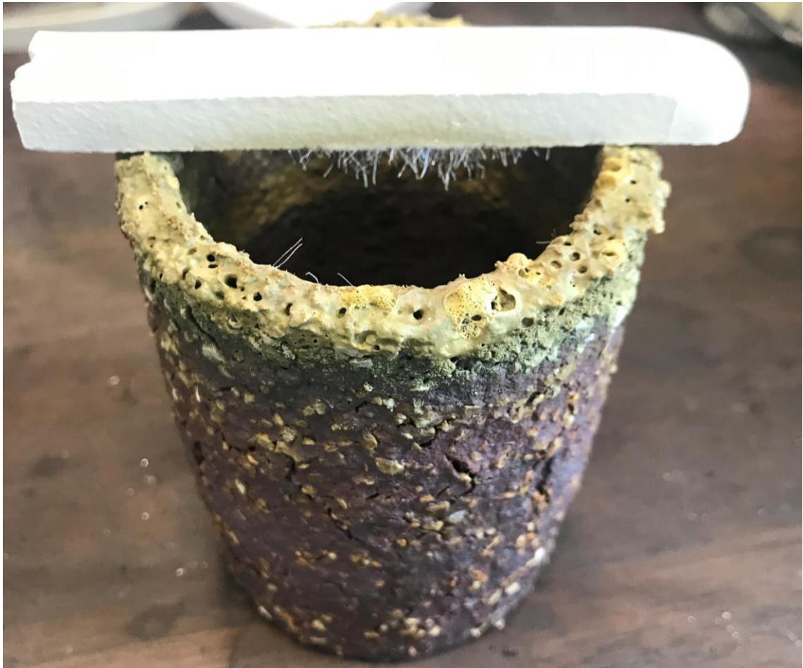
Figure 5.24. Arrangement of inverted alumina boat rested on top of Si-C crucible used to collect metal vapour in-situ.
