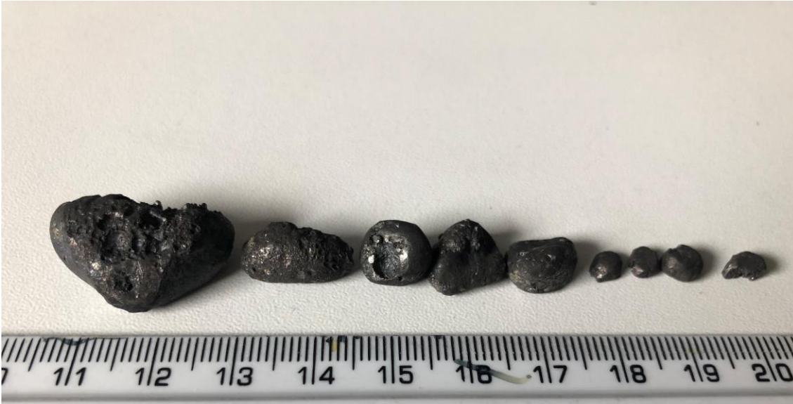
Figure 6.18. Size distribution of pig iron nuggets produced from 13.5 g briquettes.
