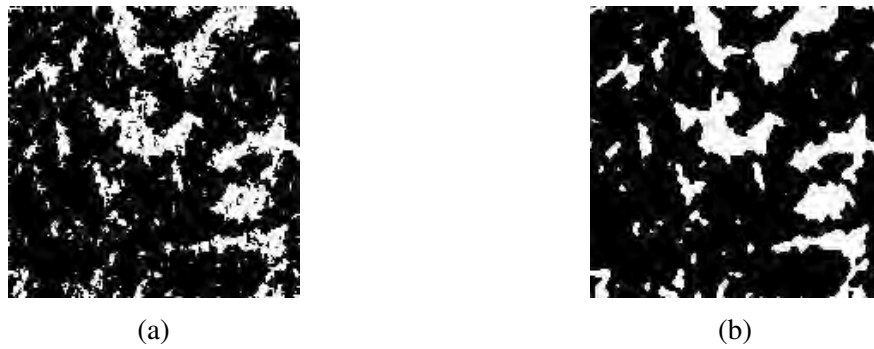
Fig. 5.6 Noise reduction and image smoothing for 2D layers in the 3D reconstructed microstructure: (a) before image processing and (b) after image processing
