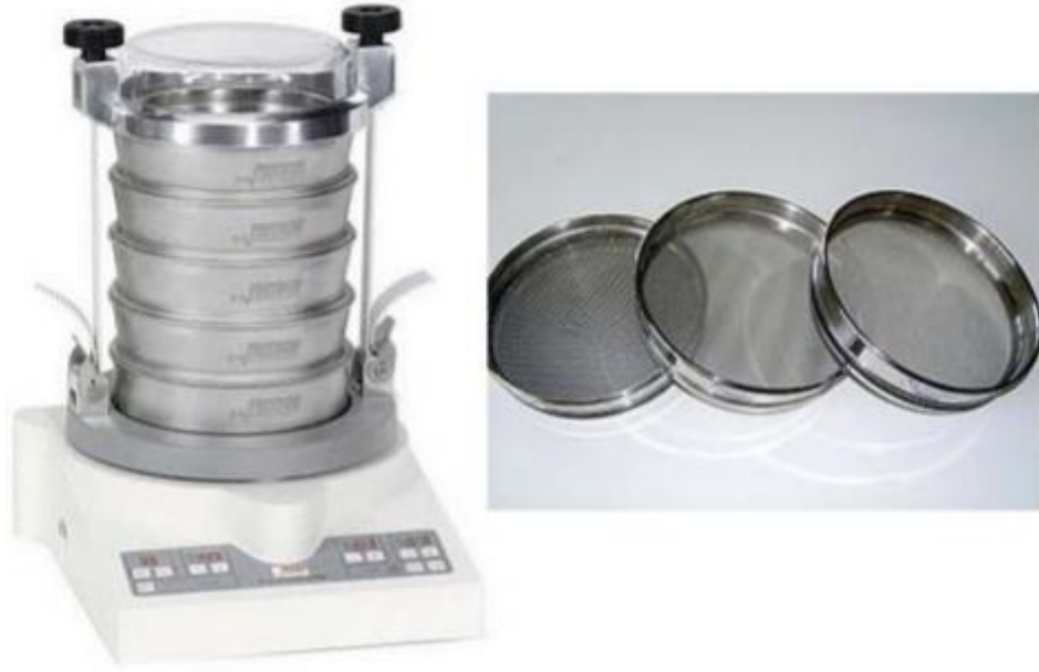
Figure 2.6: Example of a sieve shaker equipment and wire cloth sieves
