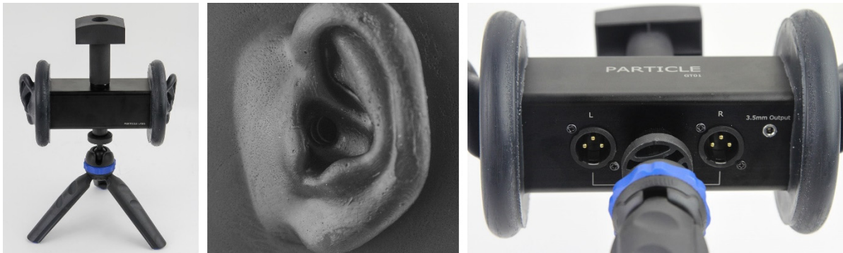
Figure 2. Custom set of artificial ears manufactured with soft silicone earmolds on either side and two IEC711 occluded ear simulators to measure the frequency response of headphones. There are both XLR and 3.5 mm microphone outputs to aid in the same.
