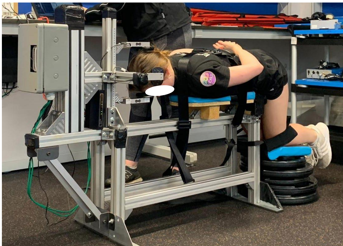
Figure 1: The neck strength test rig with a person demonstrating the required position
