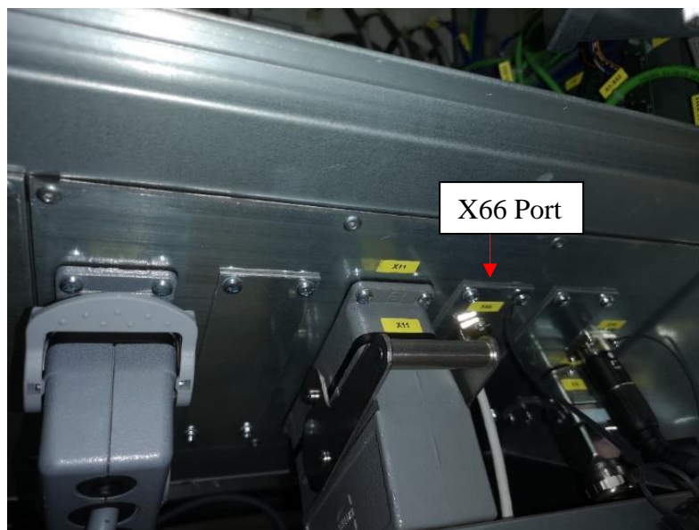
Figure 3-12 KUKA C4 cabinet X66 port location
