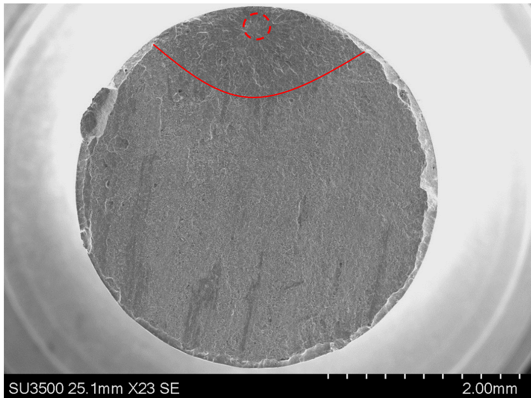
Figure 4.3.2.6: Macroscopic image of the fracture surface for the interlayer bonded HCF specimen.
