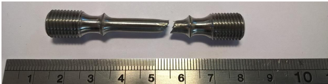
Figure 4.3.3.2: Image of fractured Tensile sample from Ti-6246 PIB.
