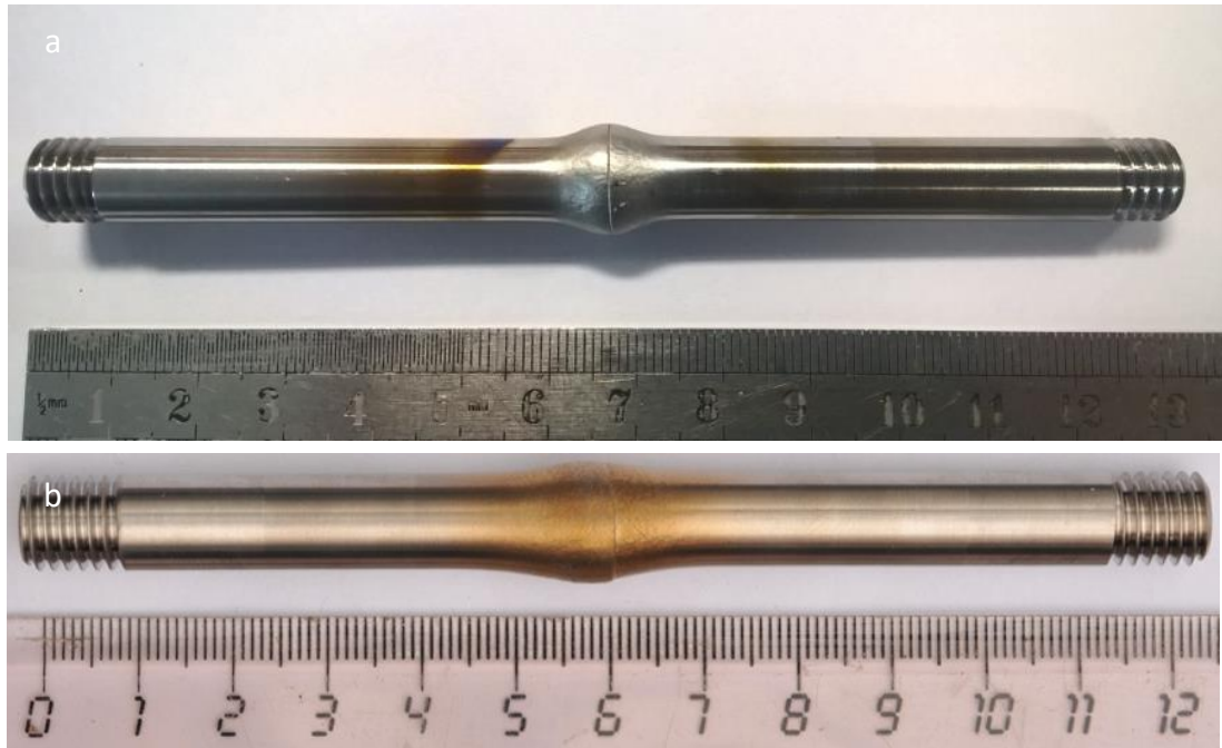
Figure 3.2.2.1: Images of Ti-6246 interlayer bonded under (a) argon shielding and (b) High vacuum
