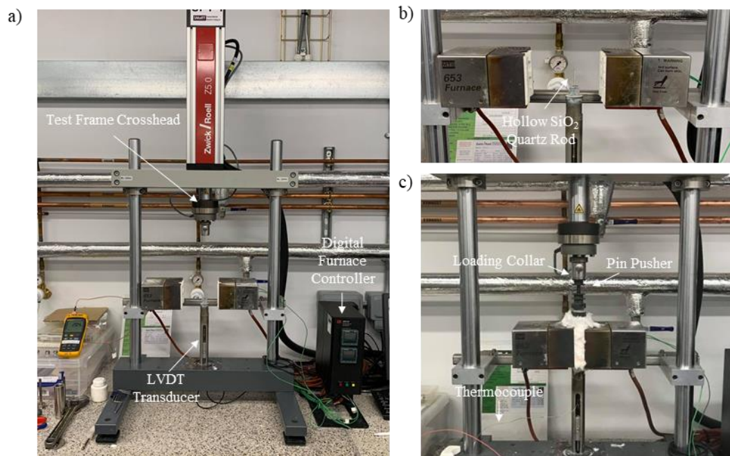
Figure 3.5. SPT setup a) Zwick / Roell Z5.0 hydraulic testing frame, b) quartz rod and c) loading collar introduced to pin punch during high temperature test.
