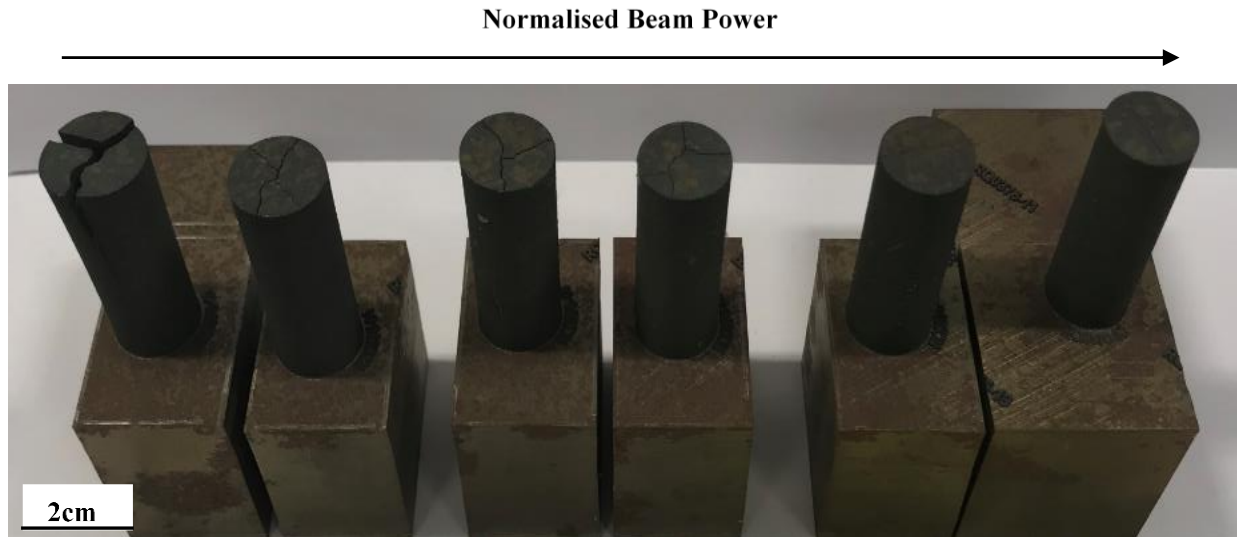
Figure 5.20. Cracking observations in LPBF CM247LC rods post HIPing from left to right in order of increasing normalised beam power.
