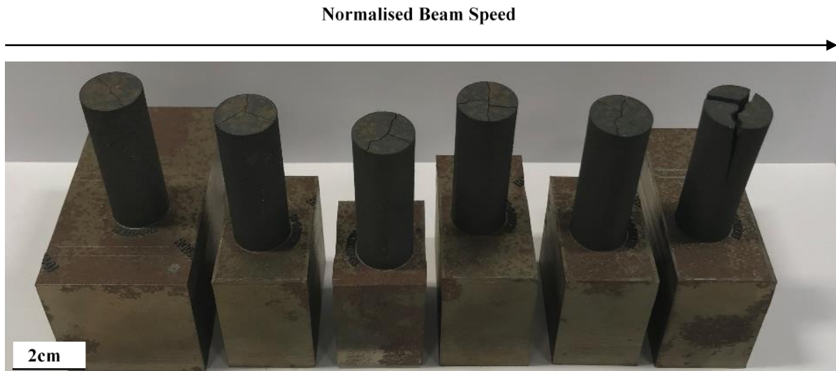
Figure 5.18. Cracking observations in LPBF CM247LC rods post HIPing from left to right in order of increasing normalised beam speed.
