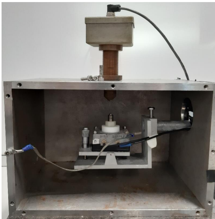
Figure 2.6 Experimental setup of the SKP apparatus
