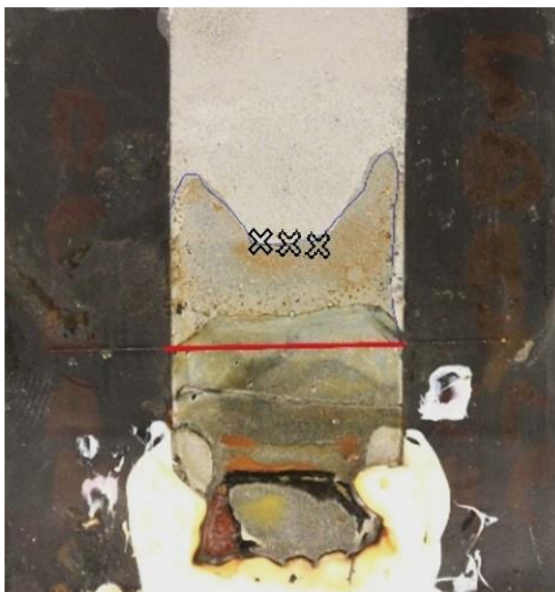
Figure 2.9 a delamination cell described in section 2.6 Where the red line is the PVB/RAPTOR interface, the white surrounding the defect is the silicon sealant and the 'x' are the points where the measurements are taken from.
