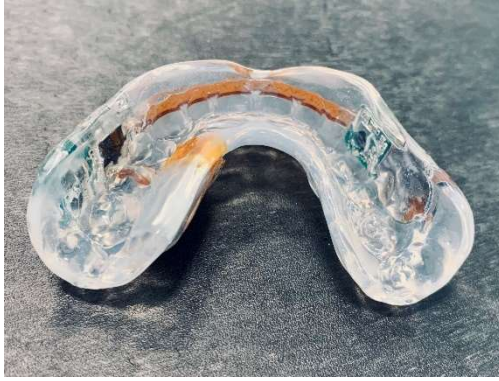
Figure 2: Electronics embedded in PROTECHT® mouthguard
