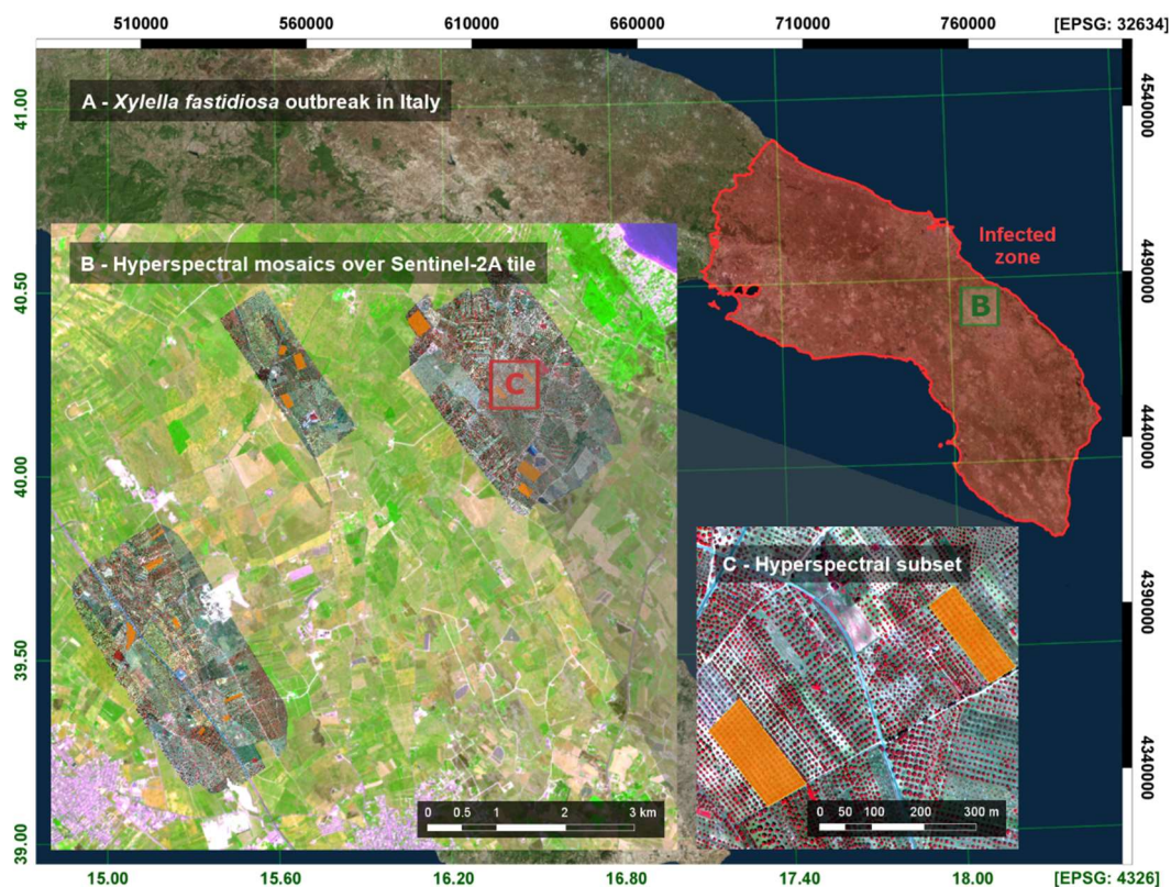
Figure 2.1 Sentinel 2A scene of southern Italy (large inset, A) with an overlay (green box, B) in which airborne hyperspectral mosaics are shown. The three hyperspectral images were acquired from aircraft on 28 June 2016 with a micro-hyperspectral imager (red box, C) yielding 40-cm spatial resolution. The infected zone highlighted in the main map (A) outlines the area where Xylella fastidiosa has been observed as of March 2018 (Commission Implementing Decision (EU) 2018/927, 2018)
