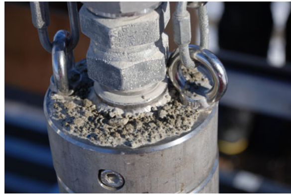
Fig. 4. Sediments on the drill stem after removing the drill from the hole (example from Hole 3).
