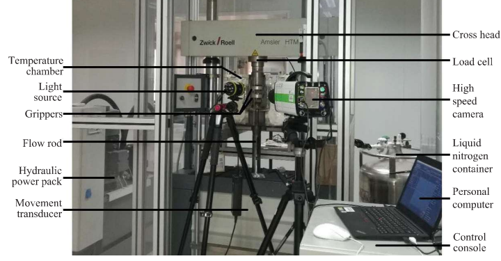
Figure 1: Zwick/Roell HTM-2512 servo-hydraulic tensile machine and a high speed camera.
