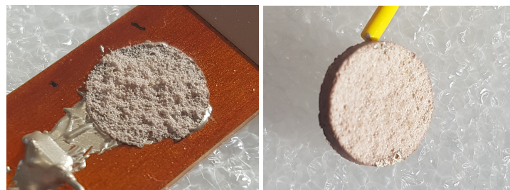
Figure 5. Test 9 which detached during the dynamic experiment.
