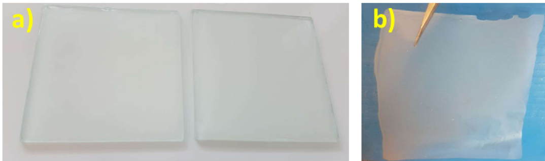
Figure 1: (a) PVA-NC-nano zeolite-Y solution being cast and dried on a glass slide (b) PVA-NC-nano zeolite-Y membranes after drying and peeled off from the glass slide.
