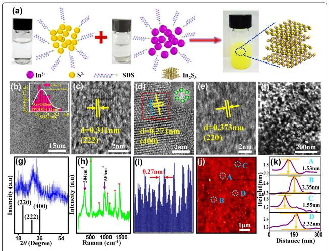
**Fig. 1** a The schematic illustration of the preparation of  $\ln_2 S_3$  QDs. b TEM image and size distribution (inset) the white line is the Gaussian fitting curve. c-e HRTEM images, inset of FFT image of a selected red area. f The SEM image. g XRD spectrum. h Raman spectrum. i The line profile of the diffraction fringes in (d). j The AFM image. k The height analysis of randomly selected  $\ln_2 S_3$  QDs labeled as A, B, C, and D in j
