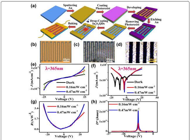
**Fig. 3** a Schematic diagram illustrating the fabrication process of the  $ln_2S_3$  QDs UV photovoltaic detector. **b** Electrode without QD. **c**–**d** Optical microscopic images of the  $ln_2S_3$  QDs photodetector at different magnifications. **e**–**h** Performance of the  $ln_2S_3$  QDs detector. **e** *J-V* curves. **f** Log (*J)-V* curves. **g** R (responsivity)-V curves. **h**  $D^*$
