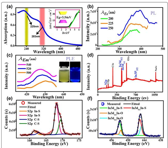
**Fig. 2** a UV-vis absorption spectra of  $\ln_2 S_3$  QDs aqueous solution. Inset: an estimation of band gap energy ( $E_g$ ). **b** PL emission spectra. **c** PL excitation (PLE) spectra, inset: luminescence image under visible and 365 nm light source. **d** The XPS full-scan spectrum. **e** XPS S2p spectrum. **f** XPS  $\ln_3 S_{3/2}$  and  $\ln_3 S_{5/2}$  spectrum
