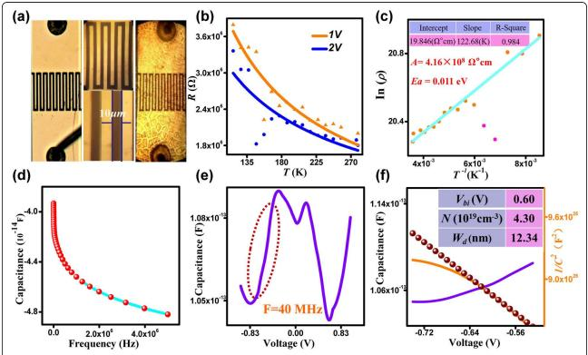
Fig. 4 a Photodetector with  $In_2S_3$  QDs as an active layer. **b** Plot of R-T at 1 V and 2 V. **c** Plot of In ( $\rho$ )-1/T-based devices at 1 V. **d** C-F curves measured at room temperature. **e** The C-V curves (40 MHz)-based photodetector in the dark condition. **f** Variation of the capacitance with applied voltages and plots of  $1/C^2$  vs. V of the device
