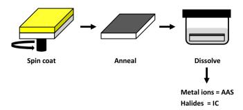
Fig. 1. Procedure to deposit, anneal and analyse perovskite films.
