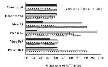
**Fig. 2.** Molar ratios of Pb<sup>2+</sup> to halide ions for tribromide, triiodide and mixed halide perovskite films spin coated onto either planar or mesoscopic TiO<sub>2</sub> coated glass substrates by 5 different researchers (R1–R5).
