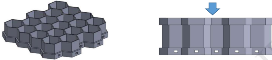
Figure 4. a) sectioned view of the honeycomb part, b) indication of load direction on part
