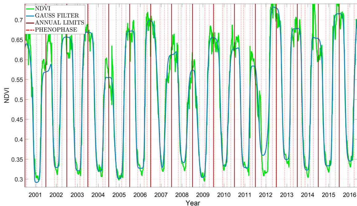
Figure 4. Moderate Resolution Imaging Spectroradiometer (MODIS) time series (2001–2016). A Gaussian filter (blue line) was applied to the original Normalized Difference Vegetation Index (NDVI) values (green line) calculated from MODIS. The red dotted lines represent the beginning and the end of each phenophase.
