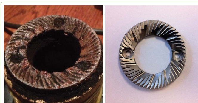
Figure 2: (a) Un-serviced grinding burr (b) New Grinding Burr.
