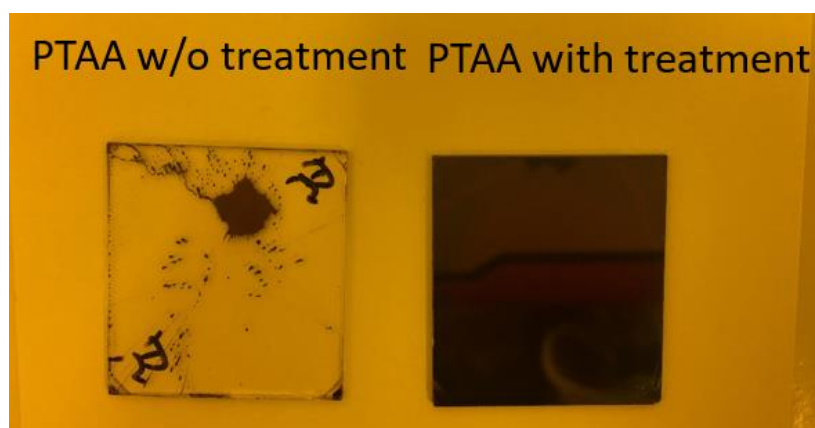
Supplementary Figure S7. Perovskite films deposited on PTAA with and without plasma treatment.
