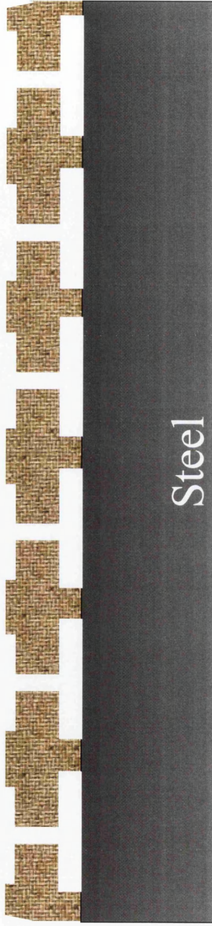
Figure 5.6 (c) Schematic of galvanized coating ( 80\text{ gm}^{-2} ) laterally sectioned
