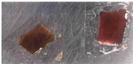
Figure 6.4: Isolation test showing the effects of either \text{Co}^{2+} or \text{Co}^{3+} species on the Fe substrate
