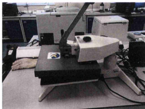
Figure 2.18: Hot press used for sealing substrates using thermosetting polymer gaskets
