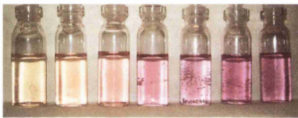
Figure 6.18: Photograph of the solvatochromic behaviour of PFPT in acetone/water mixtures: Solvent composition from left to right acetone:water; 90:10, 80:20, 60:40, 50:50, 40:60, 20:80, 10:90.
