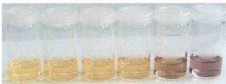
Figure 6.4: Solvatochromism of PFPT in water:THF mixtures 1 the absorption \lambda_{\text{max}} shifts from 420 nm to 540 nm with increasing water content (fig 6.3b).
