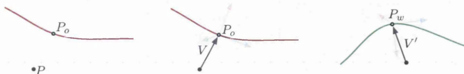
Figure 5.6: Mapping P from the object to the world wire. Note that P_o = w_o(t) and P_w = w_w(t) for the respective t -values found to minimise the distance.
