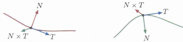
Figure 5.5: Correspondence between Frenet frames on the object wire and the world wire.
