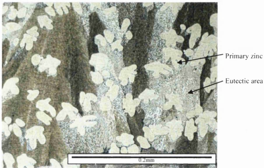
Figure 40 - polished & etched Galvalloy (ZA), 3 secs Nitpic etch
