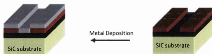
Figure 3.18 – Developing and metal deposition on the sample.
