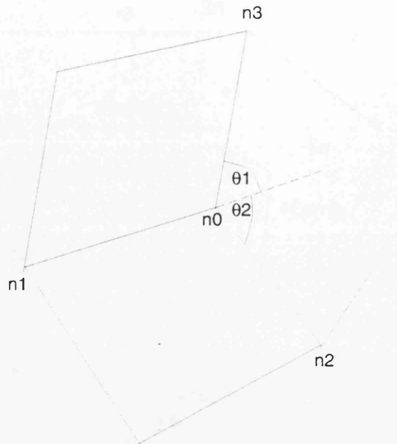
Figure 6.5: Selection of 3rd node required for monotonic slope limiting.
