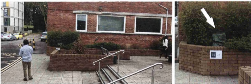
Figure 4.9: Left: A participant pointing at a sound point. Right: A close up of the sound point - a portable speaker and netbook protected by a waterproof cover. Also, a numbered label for the number entry systems.
