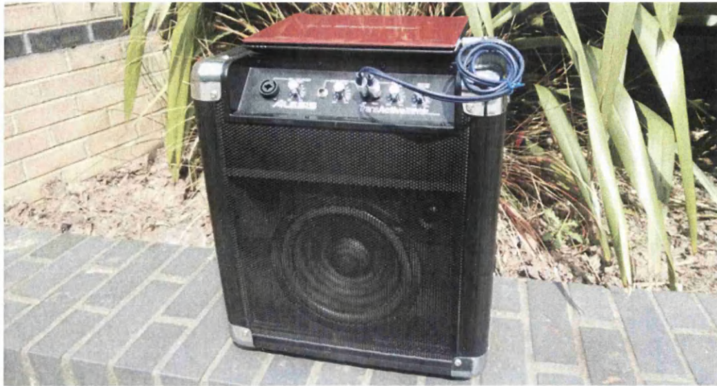
Figure 4.5: A sound point – a netbook connected to a battery powered loudspeaker. The netbook communicates with the central server via the Internet, returning the correct amplitude to play the sound through the loudspeaker.
