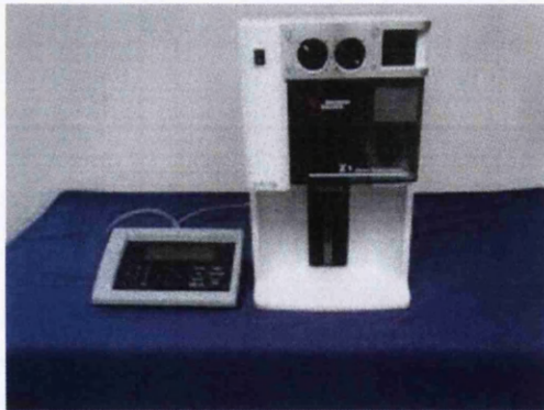
Figure 2.2 Z1 Coulter Particle Counter. Cell suspension was mixed into Coulter Isoton in the cuvette and the particles passed through the aperture their number displayed on screen. Image derived from www.bioniquet.com.uk .
