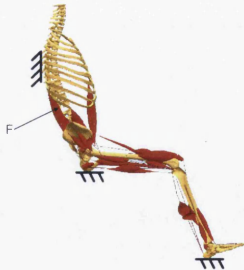
Figure 7.3: A musculoskeletal model of a seated human in the AnyBody system. The variable force F represents the lumbar support. (Rasmussen et al. [7.37])
