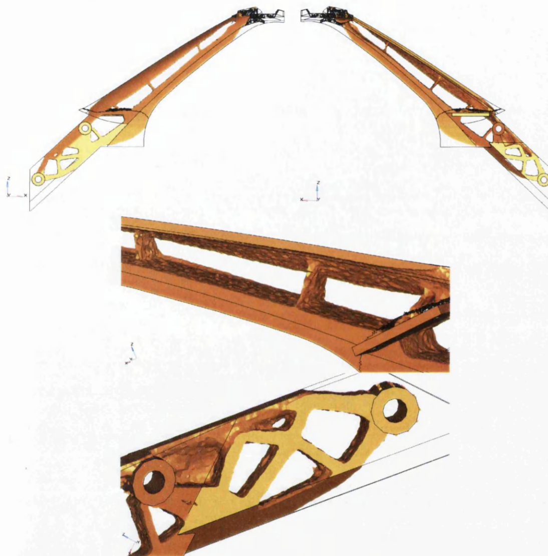
Figure 6.23: FMR7 topology optimization result from various angles for a mass target of 30%, with single and split draw direction constraints
