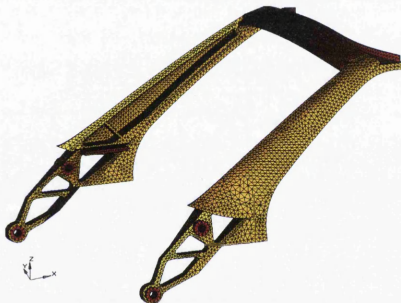
Figure 6.15: FE mesh of the manufacturable design
