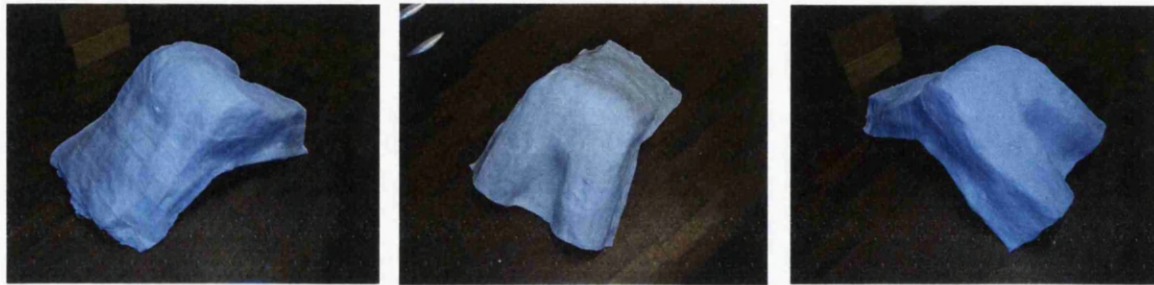
Figure 7.7: Photographs from several angles of the casting of the rigid mould developed in Section 7.3.2
