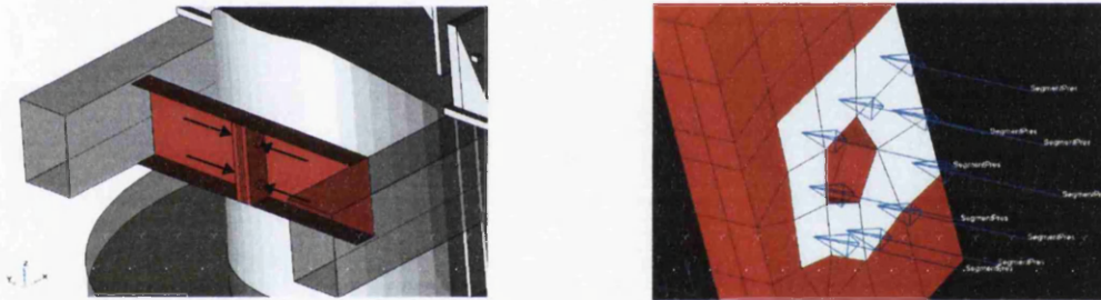
Figure 8.5: End stop clamping force: (a) location in the model; (b) force modelling
