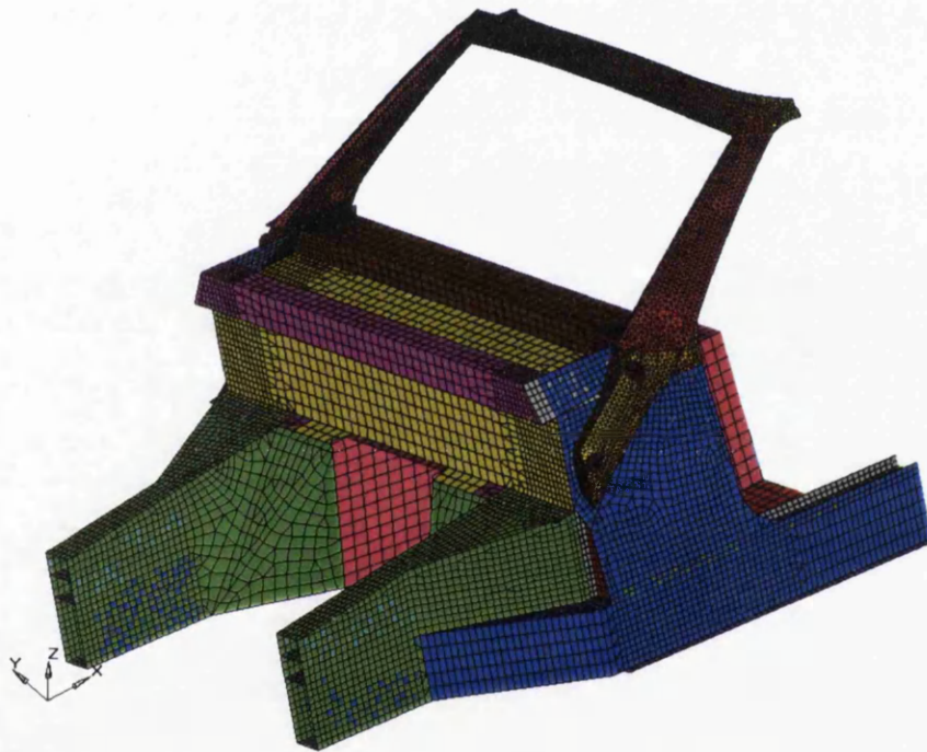
Figure 6.6: FE mesh of the model used for the topology optimization
