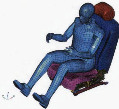
Figure 7.4: FE model of a car seat (courtesy of Jaguar Cars Ltd.) and a rigid hybrid III test dummy
