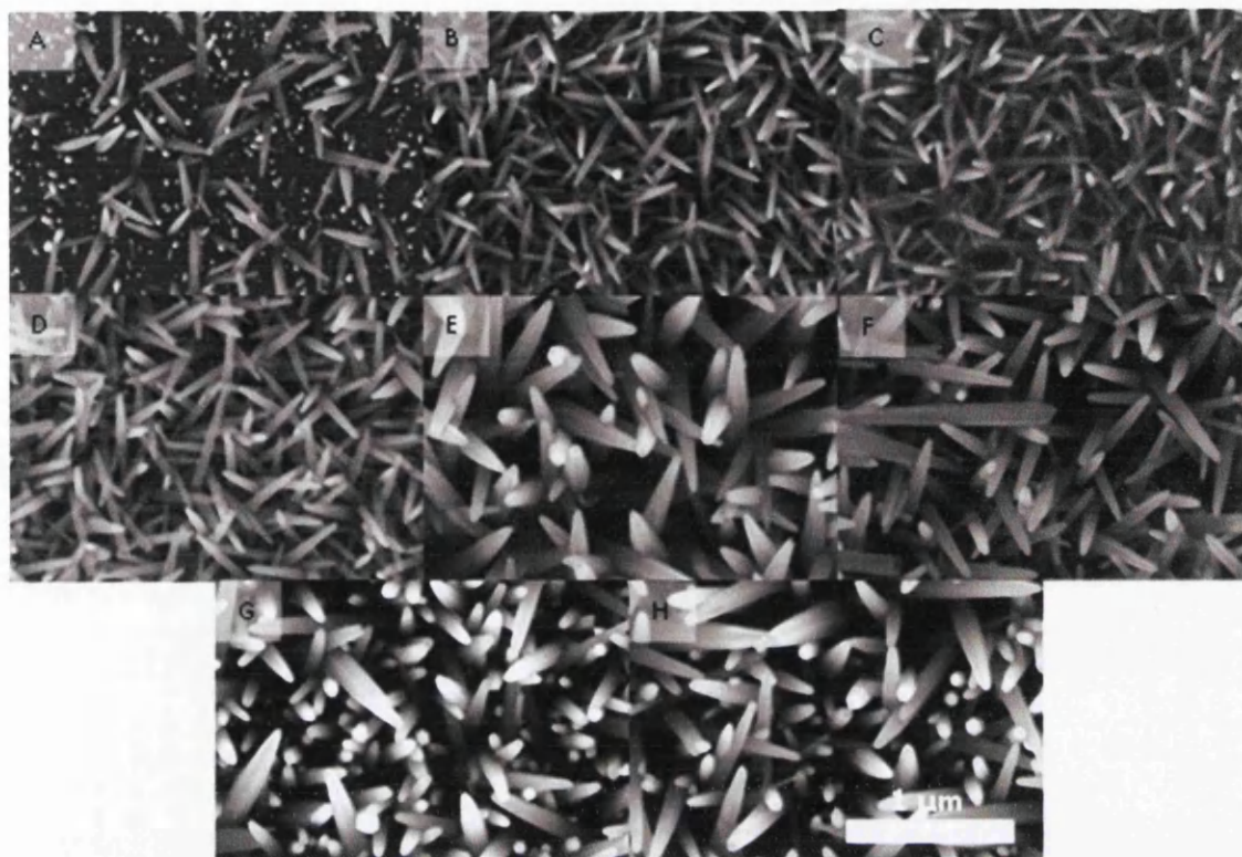
Figure 5.9: SEM images of ZnO nanowires grown aqueously in a 500ml solution containing 1.752g of HMTA and 2.126g of zinc nitrate for: A) 60 mins , B) 120 mins , C) 180 mins, D) 240mins, E) 300 mins, F) 360 mins, G) 420 mins and H) 480 mins.
