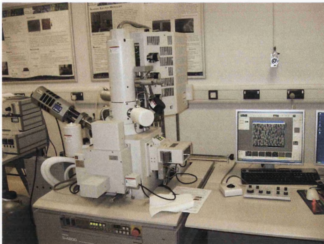
Figure 3.18: Hitachi S4800 SEM with EDX X-ray detector at Swansea University.
