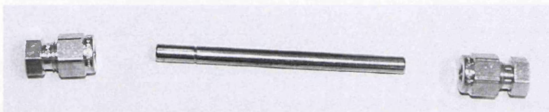
Figure 7.5: The 2-bedded thermal desorption tubes
