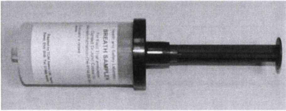
Figure 7.3: Bio-VOC ® breath sampler
