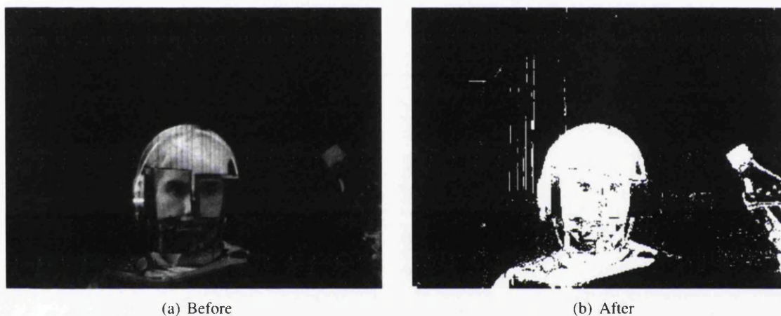
Figure 6.8: Difference in images after applying a threshold of 15
