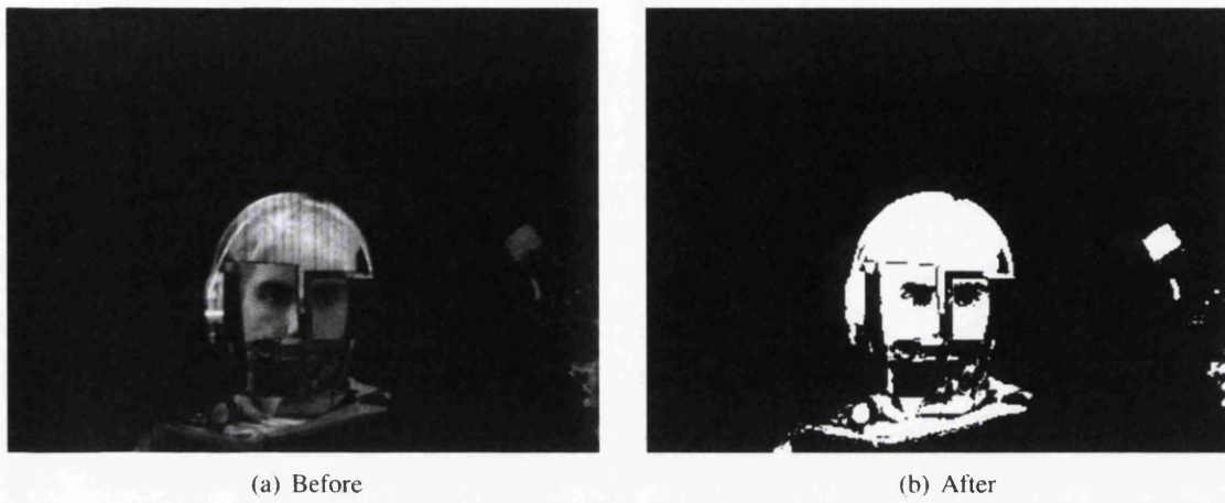
Figure 8.11: Difference in images after applying a threshold of 50
