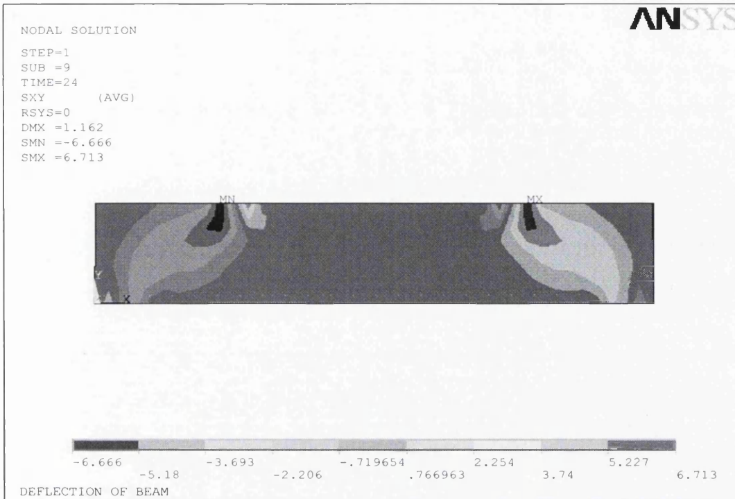
Fig. 27 Shear stress contour for Beam type 4
