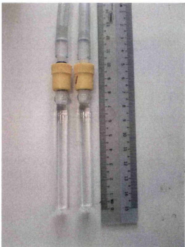
Figure 6.8 Photograph of yellow capped modified Berthelot tubes
