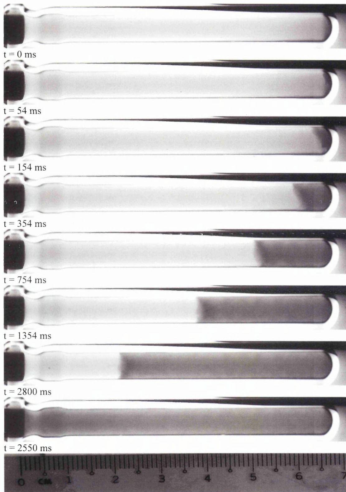
Figure 6.21 Superheated ices produced from doubly metastable orange squash in the improved Berthelot tube at -12 °C. The high-speed video system was operating at 500 frames per second (f.p.s). The velocity of the ice formation is 2.78 \text{ cm s}^{-1} .
