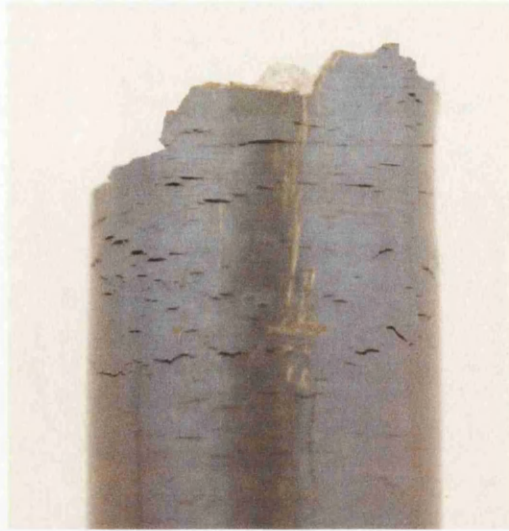
Figure 6.7 - Strain control gauge length (450°C, cyclic waveform), with multiple surface cracks
