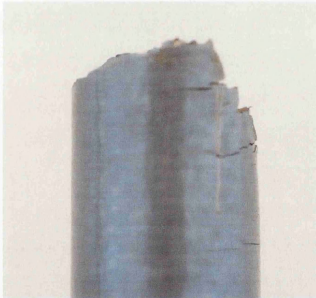
Figure 6.8 - Strain control gauge length (500°C, cyclic waveform), with multiple surface cracks
