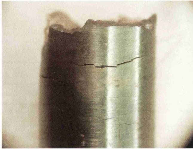
Figure 6.9: Strain control gauge length (550°C, cyclic waveform), with multiple surface cracks
