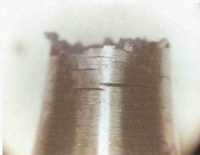
Figure 6.27 - Strain control gauge length (550°C, 2 min dwell in tension and compression), with multiple surface cracks
