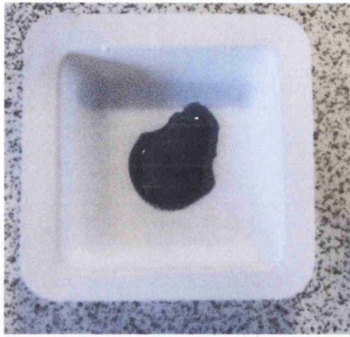
Figure 2.1. Wet blend of PSA (Styccobond F46) and PEDOT:PSS (Agfa EL-P3145)
