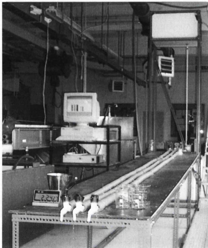
Figure 2.51. Lead pipe rig.
