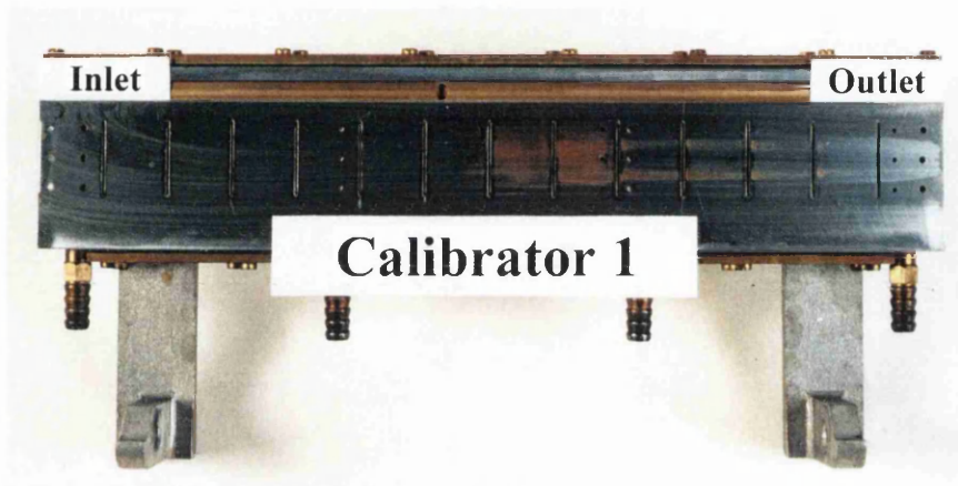
Figure A 1: Initial design of the top of calibrator 1 with holes for profile surface temperature and vacuum measurements
