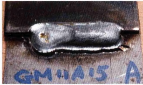
Figure 11.23: Typical Failure Location of Variable Amplitude Block Loading GM11A
