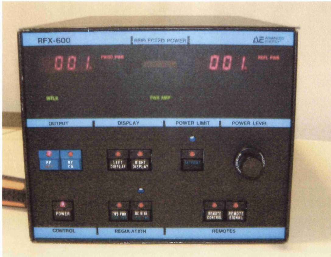
Figure 4.14(a): Advanced Energy RFX-600 RF generator
