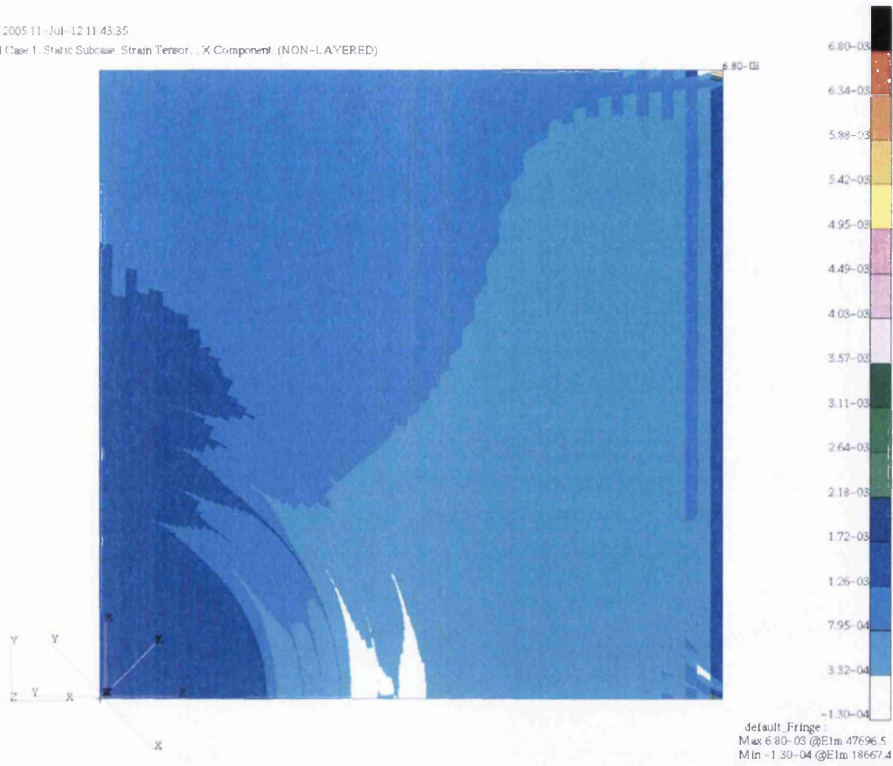
Figure 14-4: Tensile x strain of an unrepaired 3D panel
