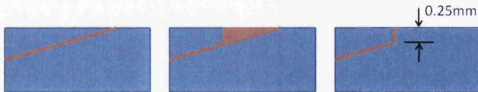
Figure 9-18: Edge tip geometries: plain; trimmed and adhesive filled and butt edge tip
