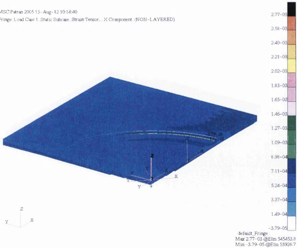
Figure 14-16: Isotropic view of the tensile x strain in the scarf region of the repair with edge elements removed
