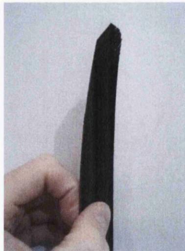
Figure 5-6: Effect of 'feathering' on scarf tip region of a composite adherend
