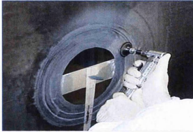
Figure 3-19: Scarf being machined out by hand [44]
