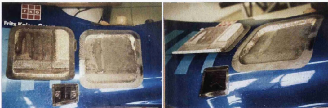
Figure 3-11: Pre-cured repair patch prepped and ready for application [53]
