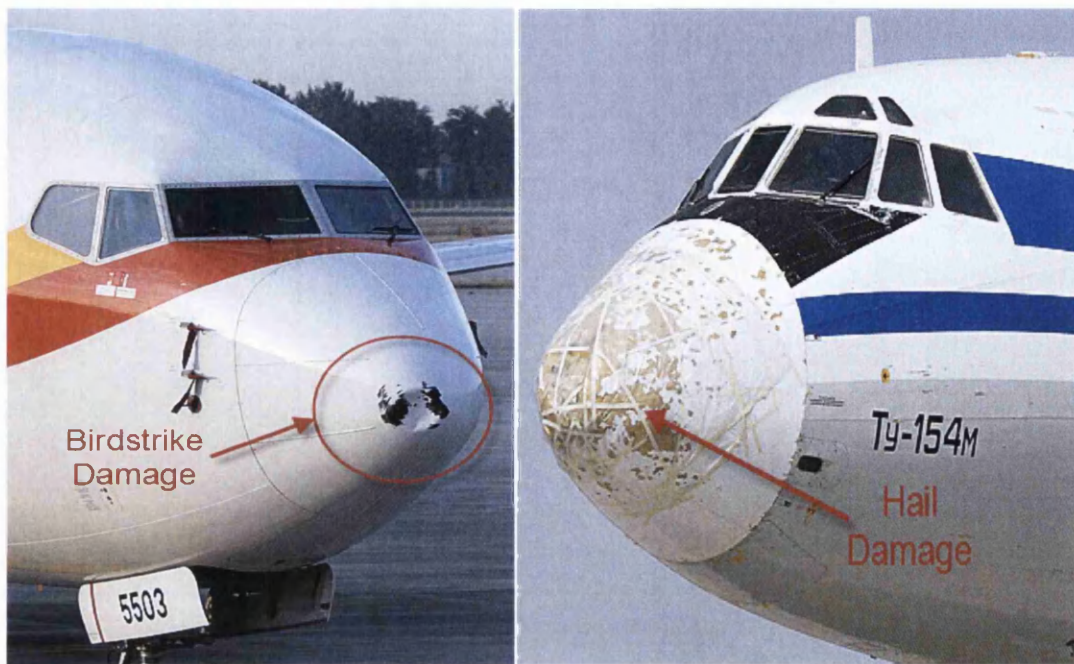
Figure 2-3: Impact damage from Bird strike and Hail [15, 16]
