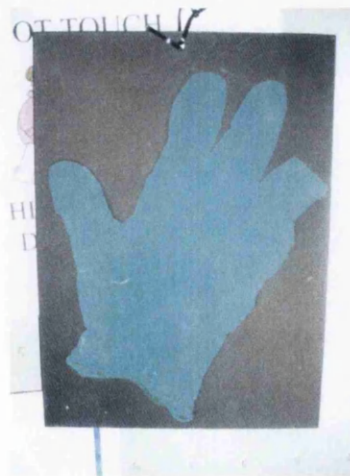
Figure 2-5: Example of FOD encountered in Manufacturing, a latex glove accidentally incorporated into a composite laminate
