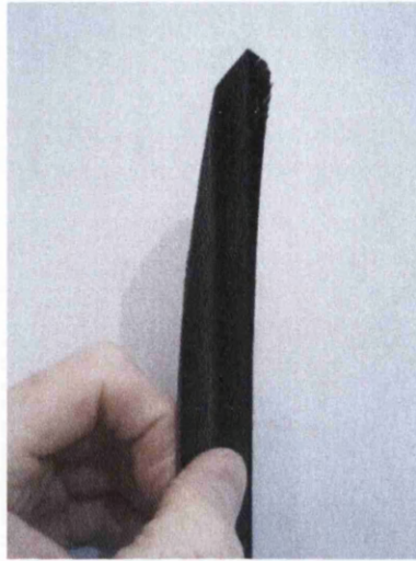
Figure 8-6: Effect of 'feathering' on scarf tip region of a composite adherend
