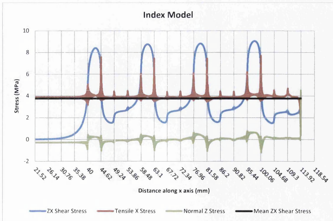
Figure 10-13: Stress profile of the bondline shear stress in a partial depth repair
