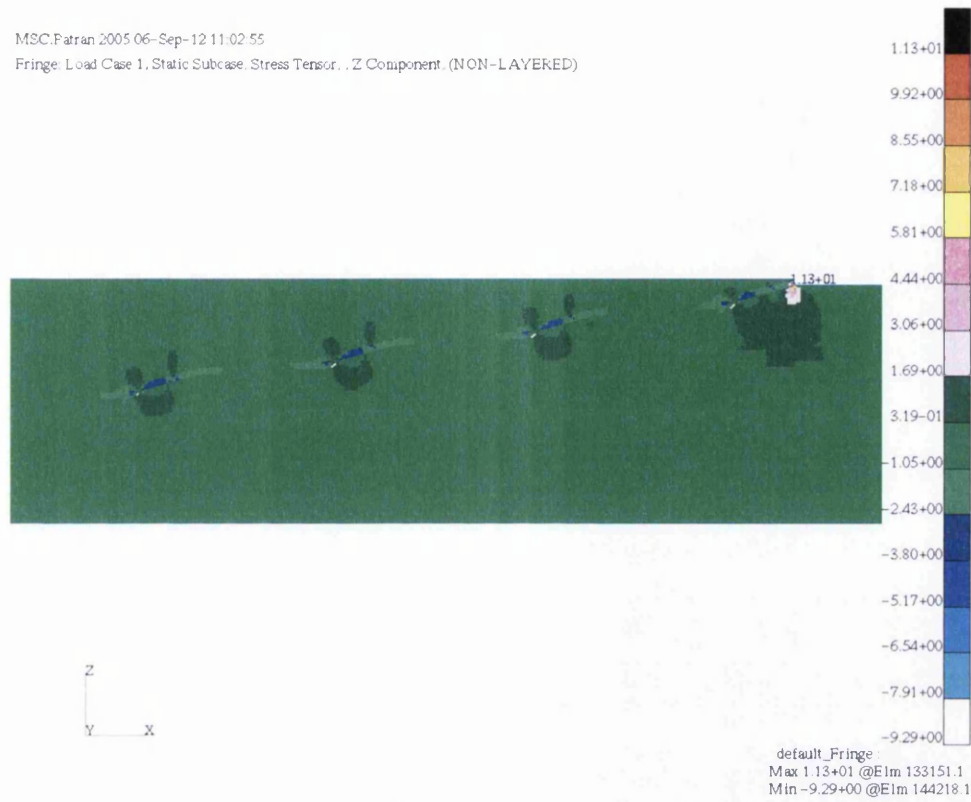
Figure 13-39: Fringe plot of the peel z stresses seen in the bondline region of the Multi-Angle concept
