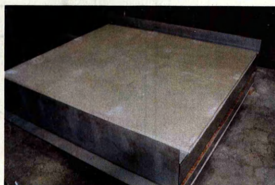
Floor and ceiling with 21mm gap
