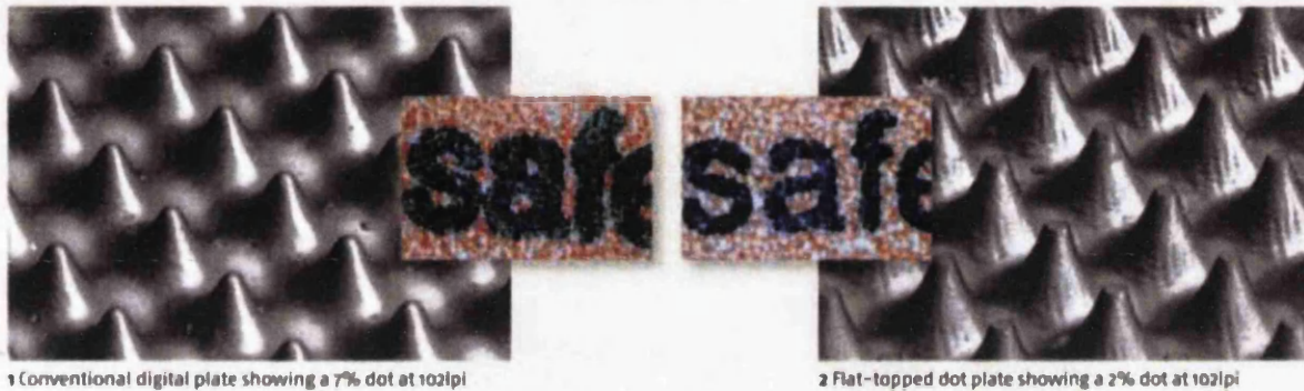
Figure 2.6: Comparison of microphotographs of standard digital (left) to “flat-topped” (right) plate features and their resultant print quality (inset pictures) (Charlesworth, 2008)
