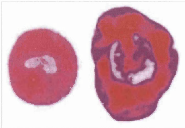
Figure 2.12: Printing defect of doughnut with approximately circular lighter area in the centre (left) and halo with crescent-shaped lighter area in the dot centre (right) (Hornschuh, 2005)
