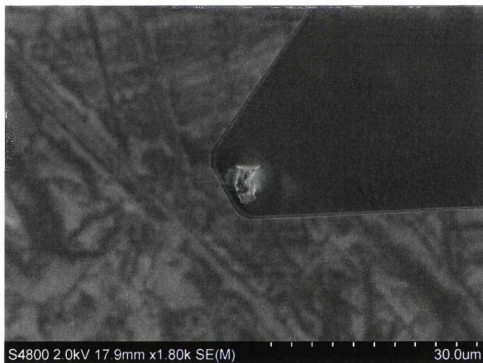
Figure 4.1. Metarhizium conidium immobilized at tip of AFM cantilever SEM image of a spore probe after force measurements.
