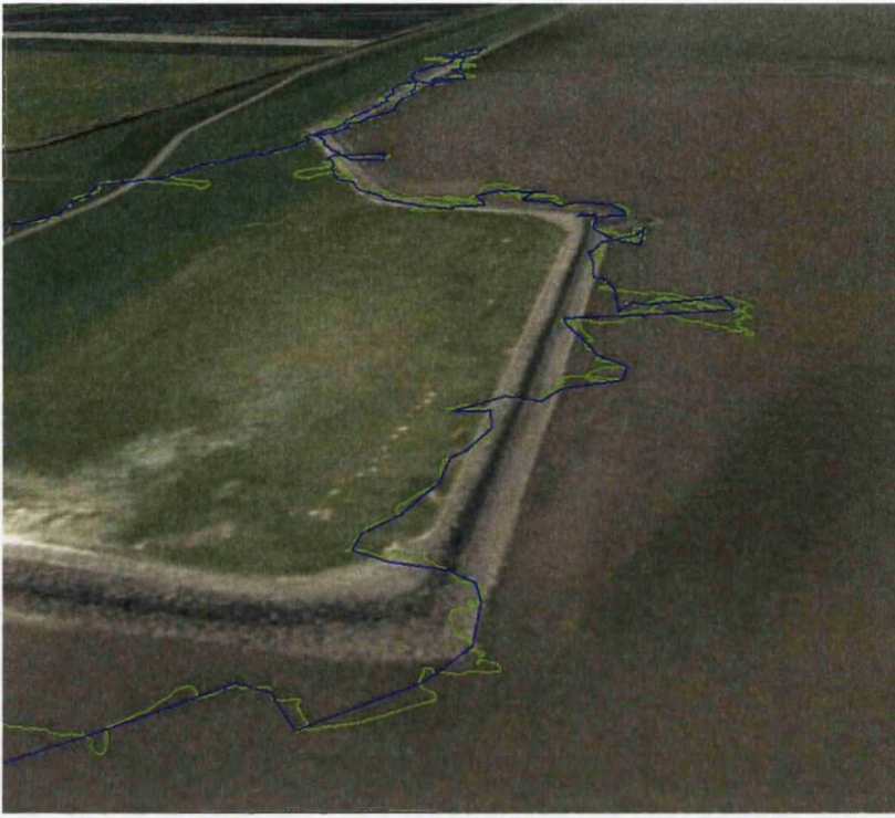
Figure 9; Movement path of a domestic dog. The purple track displays the GPS data (0.2 Hz), the green shows the path according to dead-reckoning (40Hz)
