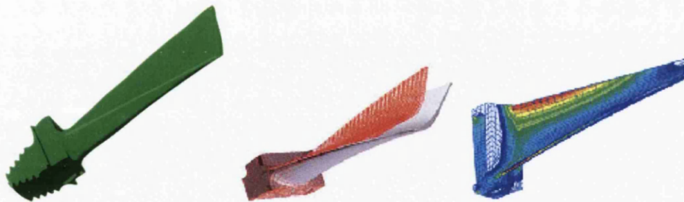
Figure 3.4: FE Analysis turbines blades. (a) Original mesh (b) deformation of blade (c) stress in the blade
